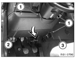
Turn rotary clips (1) through 90° and remove. Pull trim (2) downwards/backwards to remove.
